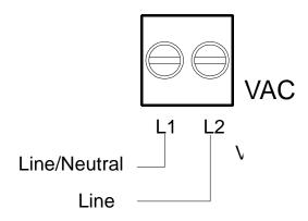
NOTE: IF ONE OF THE SUPPLY CONDUCTORS IS A NEUTRAL CONDUCTOR, THEN IT SHOULD BE CONNECTED TO TERMINAL "L1".
